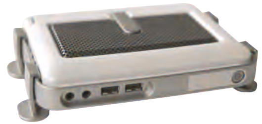
Thin-client hardware can connect users to virtual desktop VMs hosted on a secure remote server
